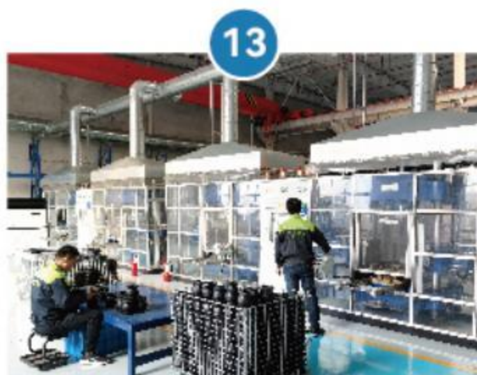
13 Inspection rubber bellow after vulcanization
