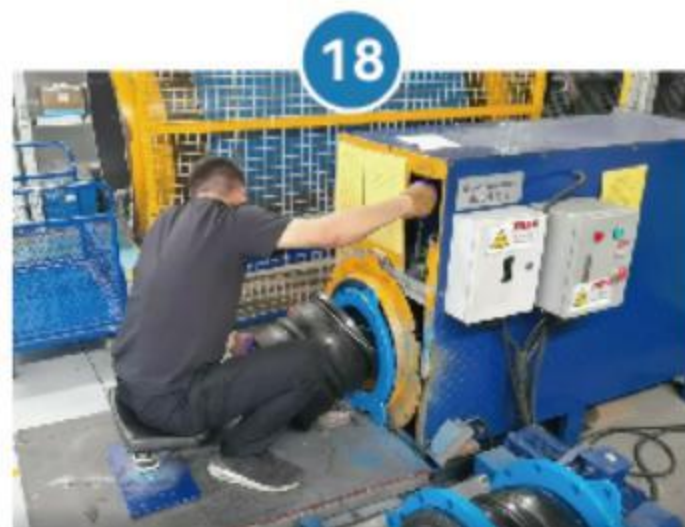
18 Assemble rubber expansion joints
