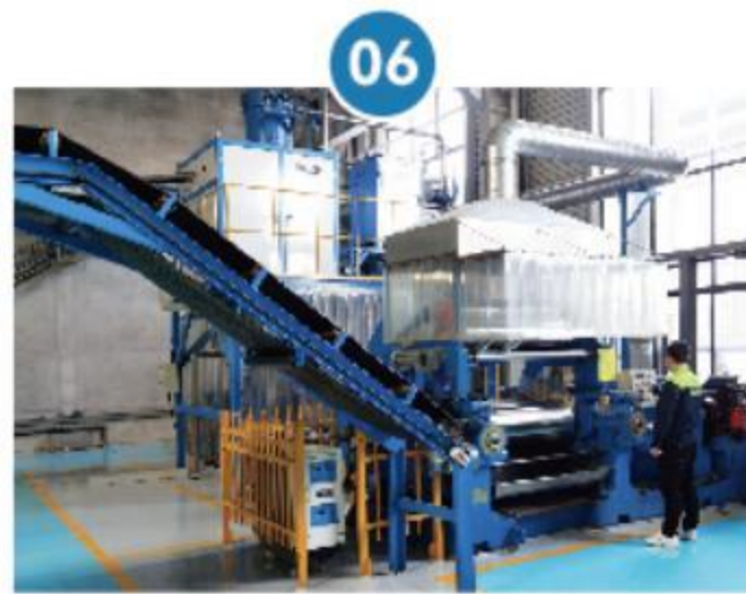
06 Banbury mixer-Mixing material compounding
