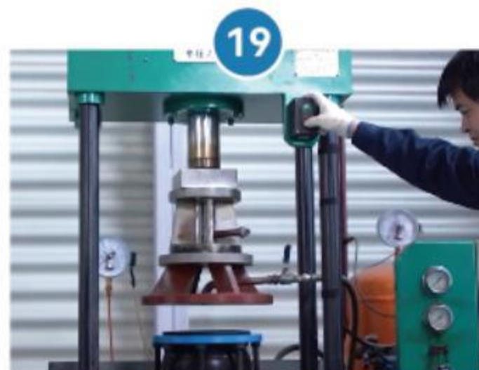
19 Rubber joint hydraulic pressure testing
