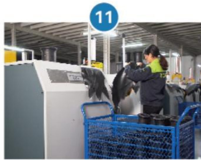
11 Automatic forming of the entire rubber bellow
