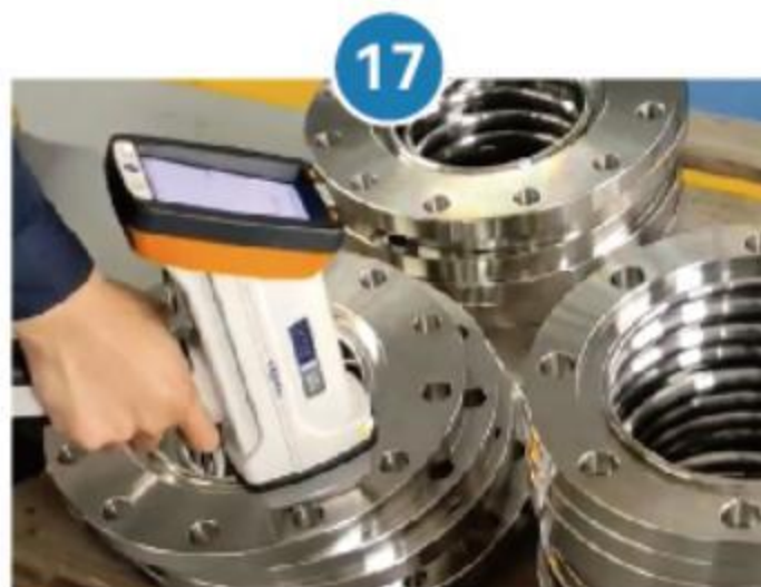
17 Flange material testing
